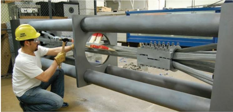
Wedges being driven into the cable sample
